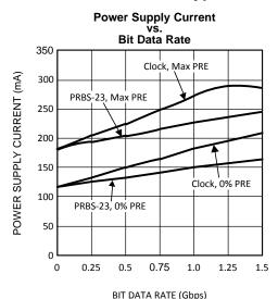
Dynamic power supply current was measured while running a clock or PRBS  $2^{23}$ -1 pattern with all 4 channels active.
