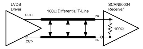
Figure 3. Typical LVDS Driver DC-Coupled Interface to SCAN90004 Input
