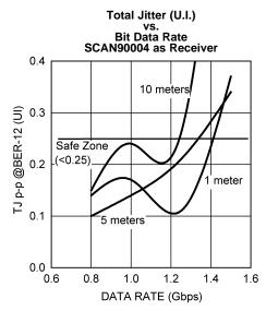
Total Jitter measured at SCAN90004 receiver outputs after receiving a PRBS  $2^7$ -1 NRZ pattern over the specified cable length.  $V_{CC} = 3.3V, \, T_A = +25^{\circ}C, \, V_{ID} = 0.5V, \\ \text{data collected at receiver outputs,} \\ \text{receiver located at end of specified Belden 1700A cable length.} \\ \text{Figure 10.}$
