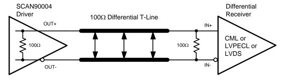
Figure 6. Typical SCAN90004 Output DC-Coupled Interface to an LVDS, CML or LVPECL Receiver
