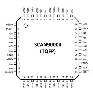
Figure 1. SCAN90004 Block Diagram
