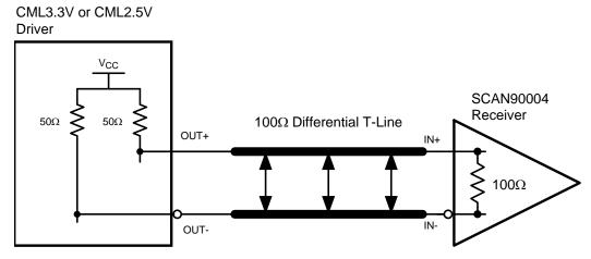
Figure 4. Typical CML Driver DC-Coupled Interface to SCAN90004 Input
