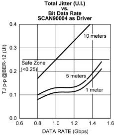
Total Jitter measured while SCAN90004 output is driving a PRBS  $2^7$ -1 NRZ pattern with a single active channel across a Belden 1700A cable.  $V_{CC}=3.3V,\, T_A=+25^{\circ}C,\, V_{ID}=0.5V,\, 0\%$  Pre-emphasis. Data measured at end of specified cable length.
